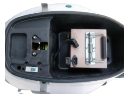
3. Disconnect Battery Power Plug Socket
